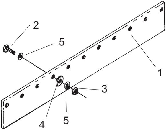
**NOTE:** The Metal mounting brackets that bolted to Deck between Deck and rubber Flaps was removed in May 1994, After tht date the Rubber Flaps bolt directly to the Deck. Qty. Shown For Left and Right Wings, For one Wing use half Qty. Shown
