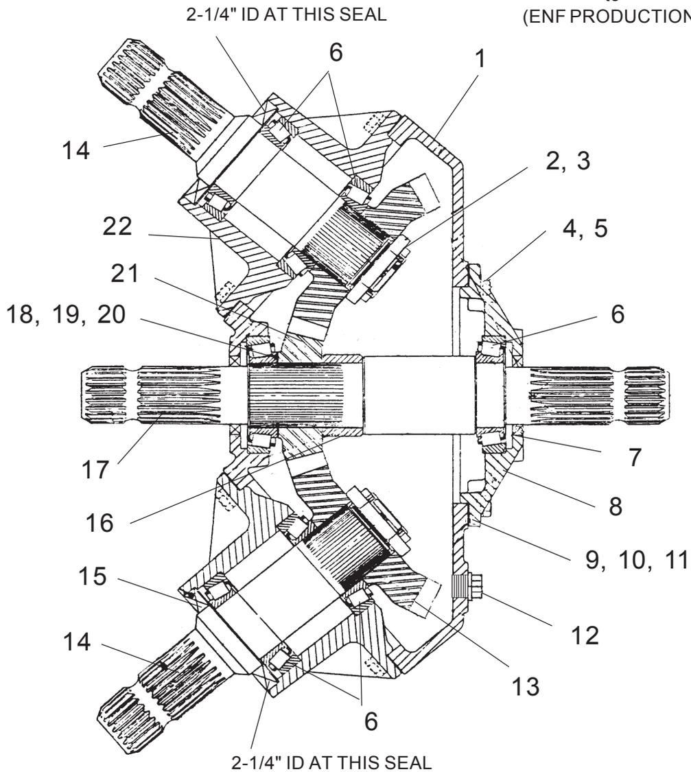
**NOTE:** To help ID this Gearbox look at Seal for Output Shaft going to the Wing Drivelines. These seals have a 1-1/4" ID and DO NOT use a Metal Seal adapter at OD of Seals, **If Gearbox looks like this but has steel adapter for Seals see the older model Gearboxes.**
