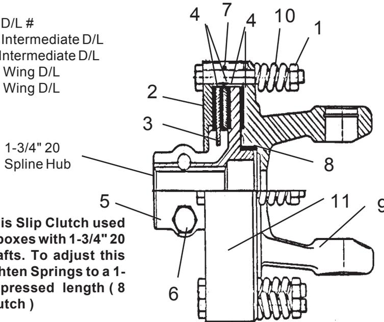
**NOTE:** This Slip Clutch used with Gearboxes with 1-3/4" 20 spline shafts. To adjust this Clutch tighten Springs to a 1-5/16" compressed length ( 8 Spring Clutch )
