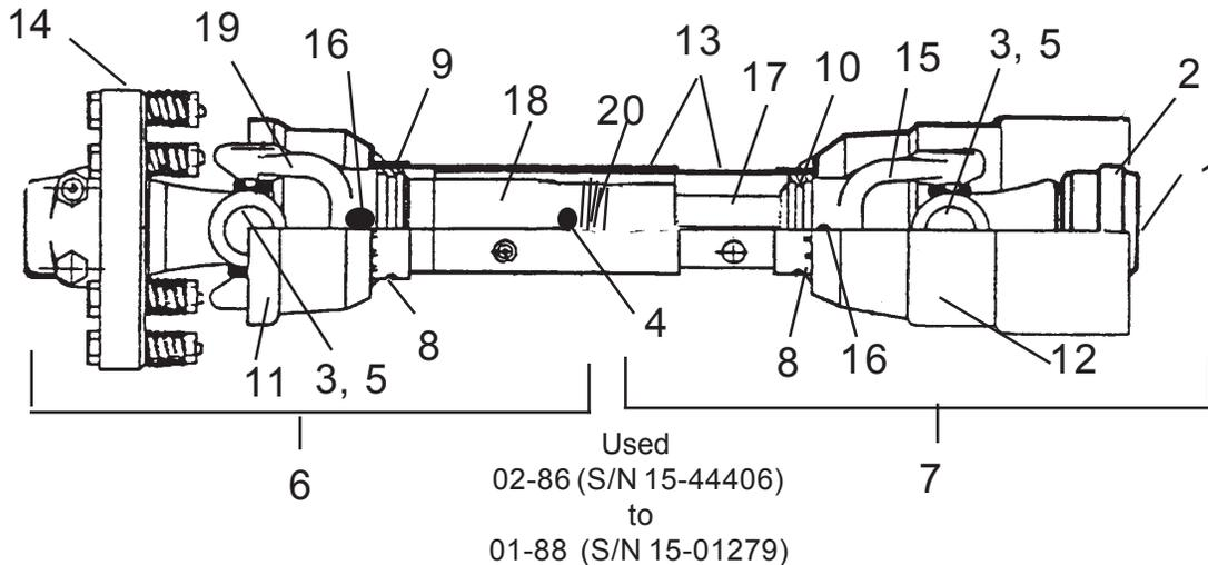
NOTE: This Driveline used with Gearboxes with 1-3/8" 6 spline shafts. To adjust this Clutch tighten Springs to a 1-5/16" length (8 Spring Clutch)
