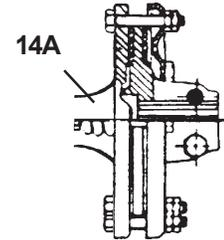
NOTE: This Slip Clutch used with Gearboxes with 1-3/4" 20 spline shafts. To adjust this Clutch tighten Springs to a 1-5/16" compressed length ( 8 Spring Clutch ). Changes were made on Item #3 and dirt Shield was removed completely from what was on earlier Serial Number Units, but main Clutch Asy Part number DID NOT Change.
