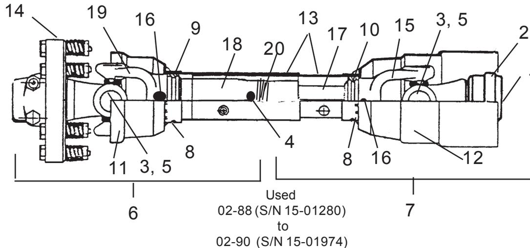
NOTE: This Driveline used with Gearboxes with 1-3/4" 20 spline shafts. A Clamp Yoke Item # 1 & 2 can be used on this D/L but WAS NOT used during production. To adjust this Clutch tighten Springs to a 1-5/16" length (8 Spring Clutch)
