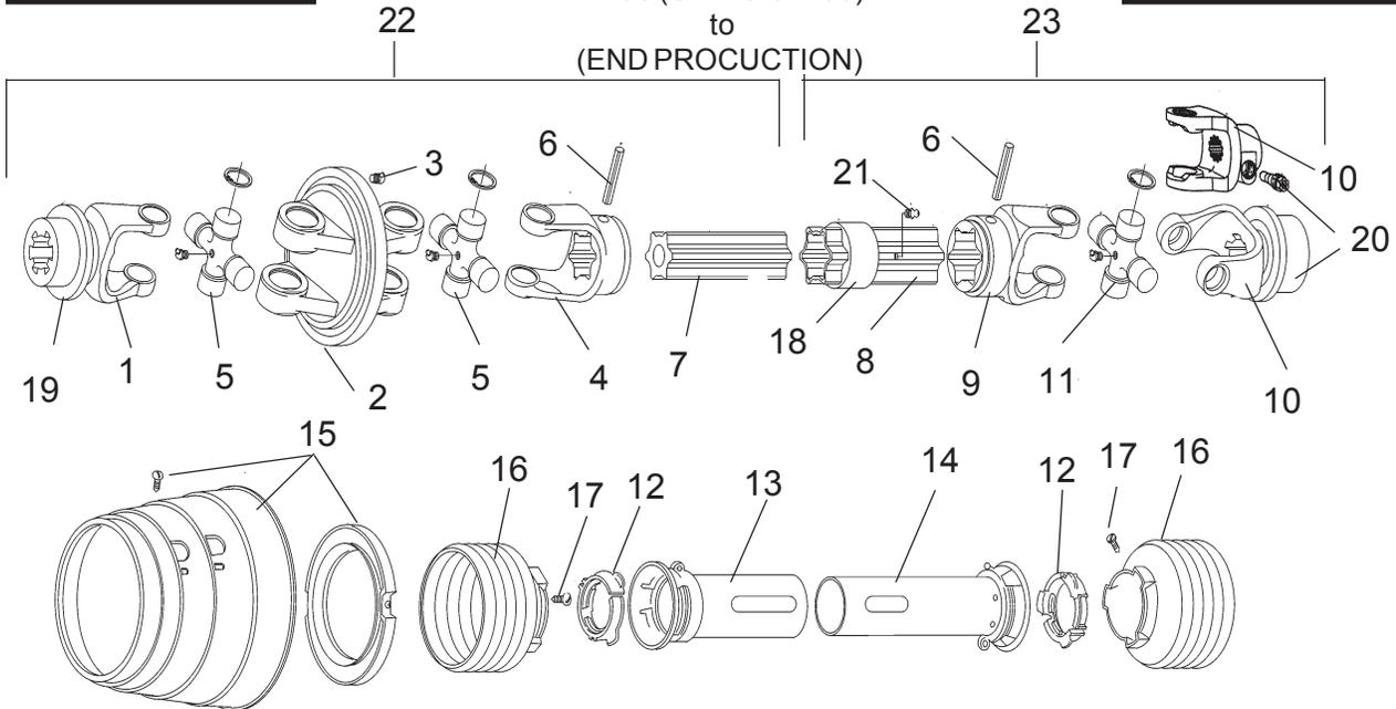
NOTE: \*\* 1-3/4" 20 spline PTO D/L is Special order Item and is longer than standard Drivelines, This D/L has 6 point Star shaped Shft & Tubes.
