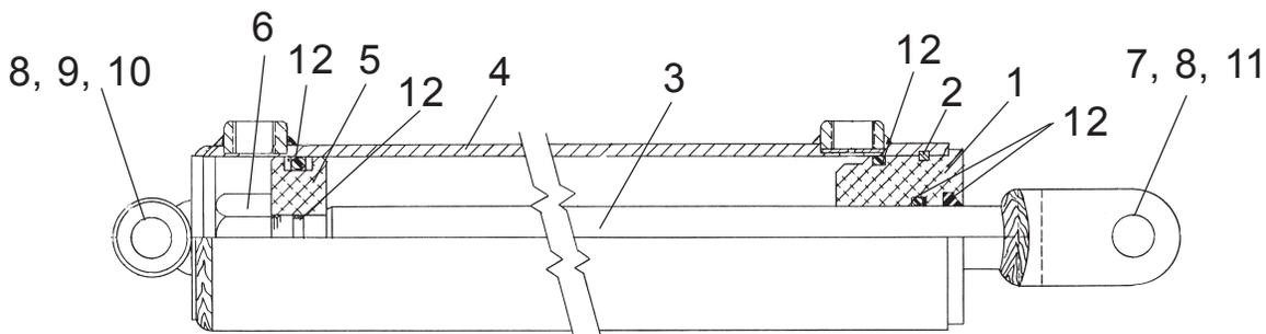
NOTE: This is a welded Cylinder Barrell (item# 4) and Gland (item # 1) is held in with a Lock Wire (item # 2). Seal Kit P/N 02841200 Includes 1 each of : Gland Static Seal, Back-Up Ring, Back-Up Rod Seal, Rod Seal, Rod Wiper, Lock Wire, Piston Seal & Rod Static Seal
