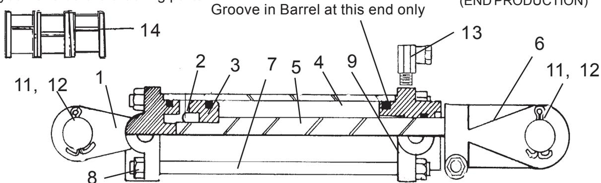
**NOTE:** Hyd Pressure **MUST** Flow from largest Cyl to Smallest, from Tractor to cylinder # 8719 to # 8720 and then to # 8721 and then back to Tractor, This System **MUST** be Purged of Air to work properly. See Hyd Chart for proper hose routing. These Cyl's **WILL NOT** work as a Standard Lift Cyl. When installing Barrels on these Cylinder grooved end **MUST** be installed at Rod end only to work properly.
