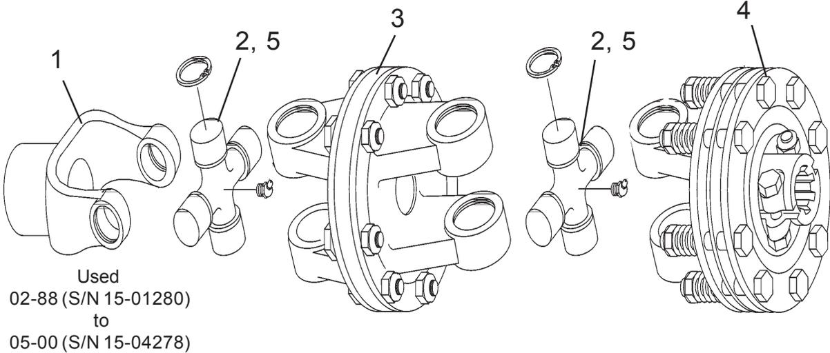
**NOTE: This Driveline used with Gearboxes with 1-3/4" 20 spline shafts. When This D/L is assembled Item # 3 MUST be bolted as shown in drawing with Yoke Ears in Time with each other for alignment. To adjust this Clutch tighten Springs to a 1-5/16" length (8 Spring Clutch). This Intermediate Driveline Assembly Cat IV (35R Equal) is replaced by new style #00775340 when replacing complete assembly, Parts WILL NOT interchange Between the old and new style.**
