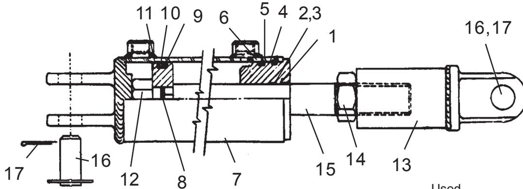
NOTE: This is a welded Cylinder Barrell (item# 7) and Gland (item # 6) is held in with a Lock Wire (item # 4)
