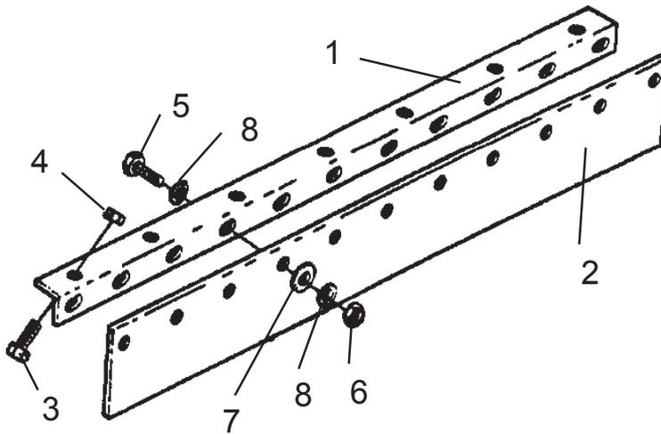
**NOTE:** Item # 1 mounting brackets were not used after May 1994, Rubber Flaps Item # 2, after that date they bolted directly to Deck. Qty. Shown For Left and Right Wings, For one Wing use half Qty. Shown
