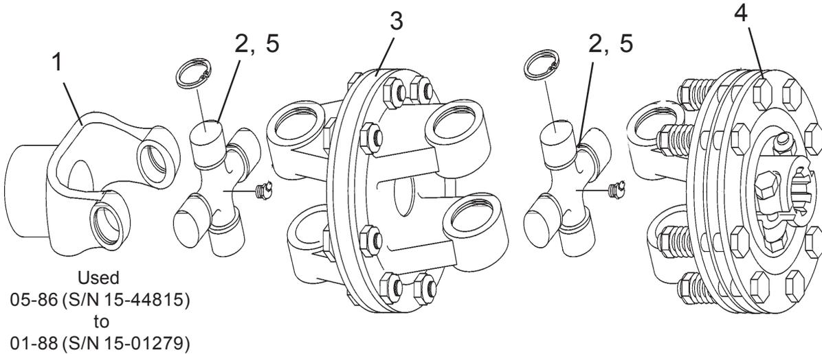
**NOTE:** This Intermediate Driveline Assembly Cat IV (35R Equal) is replaced by #00754180 when replacing complete assembly. Some Parts WILL NOT interchange, Check Part numbers to find what parts are the same. **This Driveline used with Gearboxes with 1-3/8" 6 spline shafts. When This D/L is assembled Item # 3 MUST be bolted as shown in drawing with Yoke Ears in Time with each other for alignment. To adjust this Clutch tighten Springs to a 1-5/16" length (8 Spring Clutch)**
