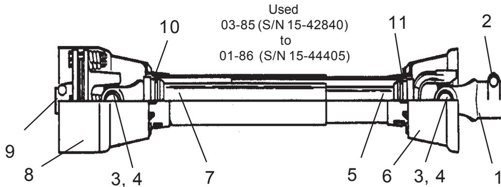
NOTE: This Driveline used with Divider Gearbox with 1-3/8" 6 spline shaft and Wing Deck with 1-3/8" 6 spline shaft. To adjust this Clutch tighten Springs to a 1-5/16" length ( 8 Spring Clutch)
