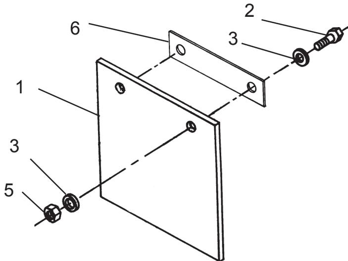
NOTE: This Rubber Flap was used with Chainguards and after July 1989 it was used with rubber deflectors, It is used on rear of Wings on inside at Hinge point. In May 1994 Nut and Lockwasher (item # 5) was replaced with a Locknut which will also work on earlier models.
