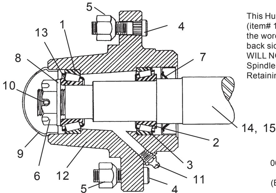
This Hub has Grease Fitting (item# 11) on Back Side and has the word Alamo cast into the back side, This Hub & Bearings WILL NOT fit on earlier S/N Spindles. This Hub used a 1" Retaining Nut (Item # 6)
