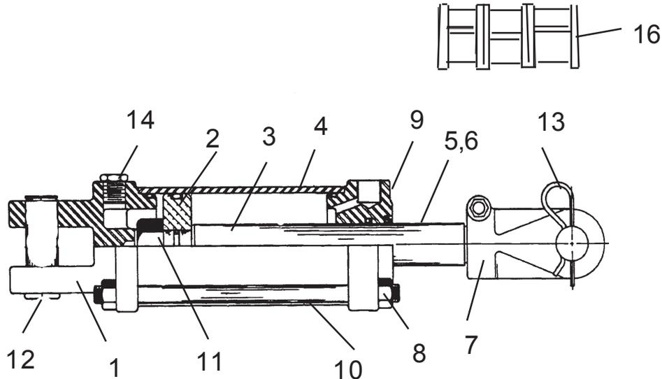
NOTE: This is a Tie Rod Cylinder (item# 10) Cylinder is held together with these Tie Rods (qty 4)
