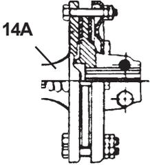
NOTE: This Slip Clutch used with Gearboxes with 1-3/4" 20 spline shafts. To adjust this Clutch tighten Springs to a 1-5/16" compressed length ( 8 Spring Clutch ). Changes were made on Item # 3 and dirt Shield was removed completely from what was on earlier Serial Number Units, but main Clutch Asy Part number DID NOT Change.
