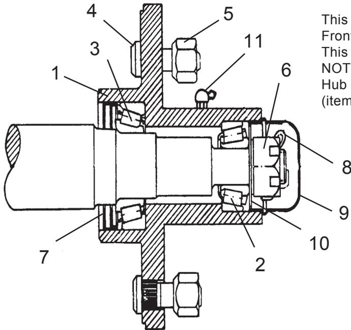
This Hub has Grease fitting on Front Side as shown in drawing, This Hub and Bearings WILL NOT fit on later S/N Spindle. This Hub used a 7/8" retaining nut (item# 6)
