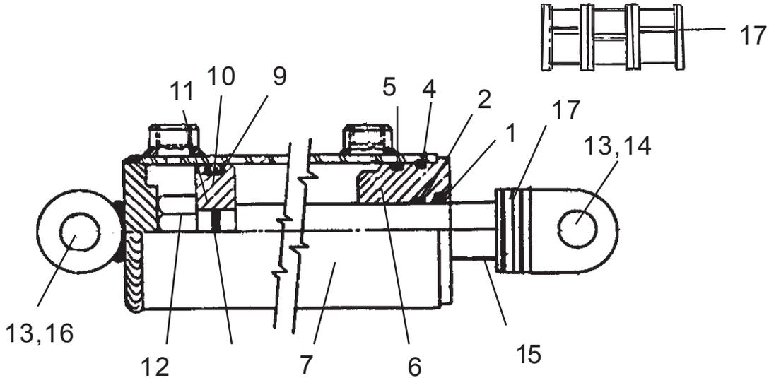
NOTE: This is a welded Cylinder Barrell (item# 7) and Gland (item # 6) is held in with a Lock Wire (item # 4)
