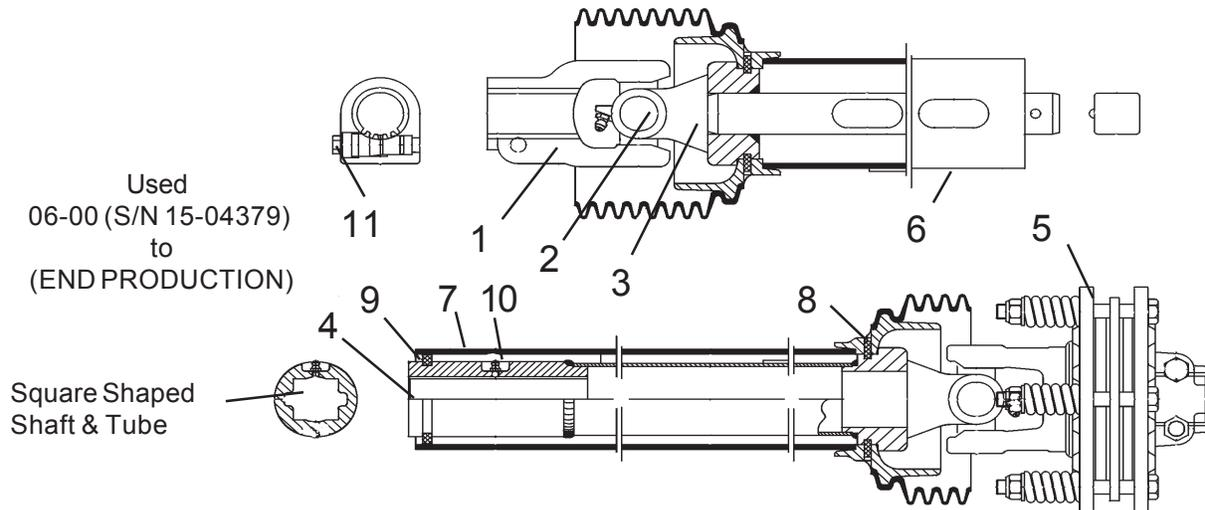
NOTE: Order parts from this page if the Tube and Shaft of your driveline has a Square shape as shown in drawing above. This Driveline used with Gearboxes with 1-3/4" 20 spline shafts. To adjust this Clutch tighten Springs to a 1-9/16" compressed length ( 6 Spring Clutch )
