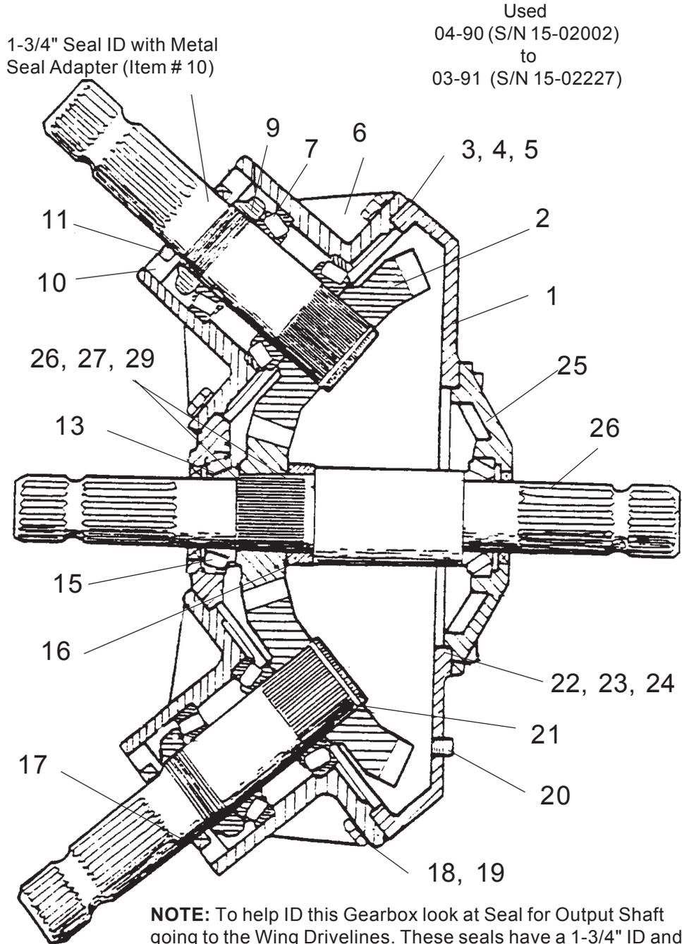
**NOTE:** To help ID this Gearbox look at Seal for Output Shaft going to the Wing Drivelines. These seals have a 1-3/4" ID and use a Metal Seal adapter (item # 10) at OD of Seals, **These Seal Adapters (item # 10) are only used on this Gearbox.**
