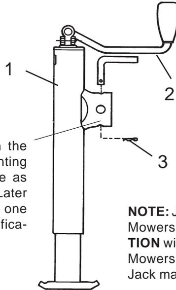
This is a shorter Jack than the previous one used but mounting lug is up high on Jack tube as shown in this drawing. This Later Jack will replace the earlier one without any changes or modifications to mount..
