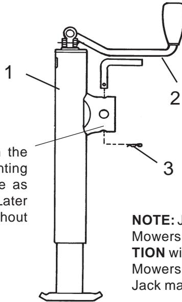
This is a shorter Jack than the previous one used but mounting lug is up high on Jack tube as shown in this drawing. The Later Jack will replace this one without any changes.
