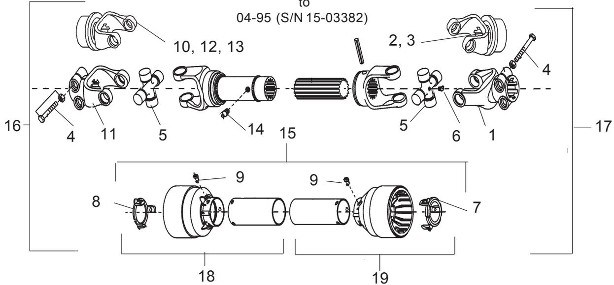
This Main D/L has Series 6 Shields. ID the new and later Series 8 D/L's by the larger Shield Tubes. The following Chart gives the Dia. & Circumference of Shields for both D/L's.
