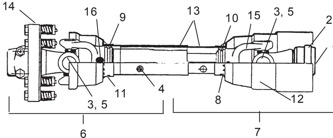
NOTE: SERIES 6 Triangle Shape Shaft & Tube with Yellow Shields, Always check Tube & Shield size before ordering Parts. This Driveline used with Gearboxes with 1-3/4" 20 spline shafts. To adjust this Clutch tighten Springs to a 1-5/16" length (8 Spring Clutch). Replace as an Asy with P/N 00757375A (with Series 8 Shields & Tubes) Some parts WILL NOT Interchange. Always Check part numbers to see which parts will interchange.
