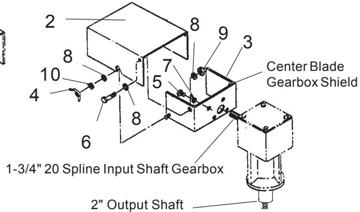
1-3/4" 20 Spline Input Shaft Gearbox
