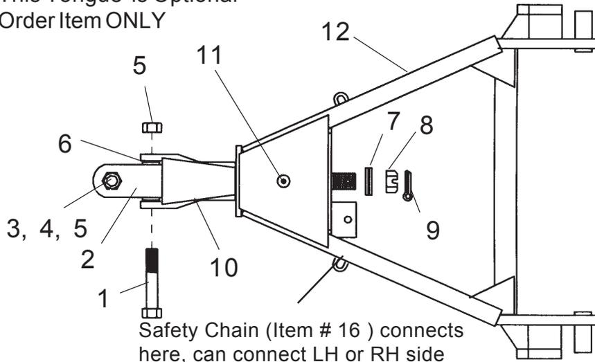
**Tongue Assembly P/N 00753574 (Dual Control Rods)**
