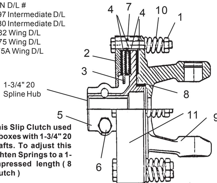
**NOTE:** This Slip Clutch used with Gearboxes with 1-3/4" 20 spline shafts. To adjust this Clutch tighten Springs to a 1-5/16" compressed length ( 8 Spring Clutch )
