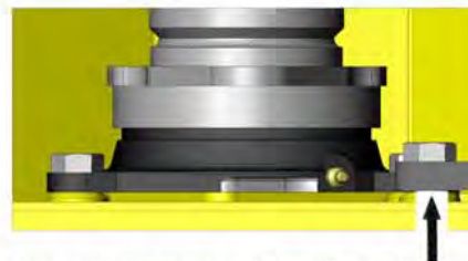
Shim where required to adjust alignment
