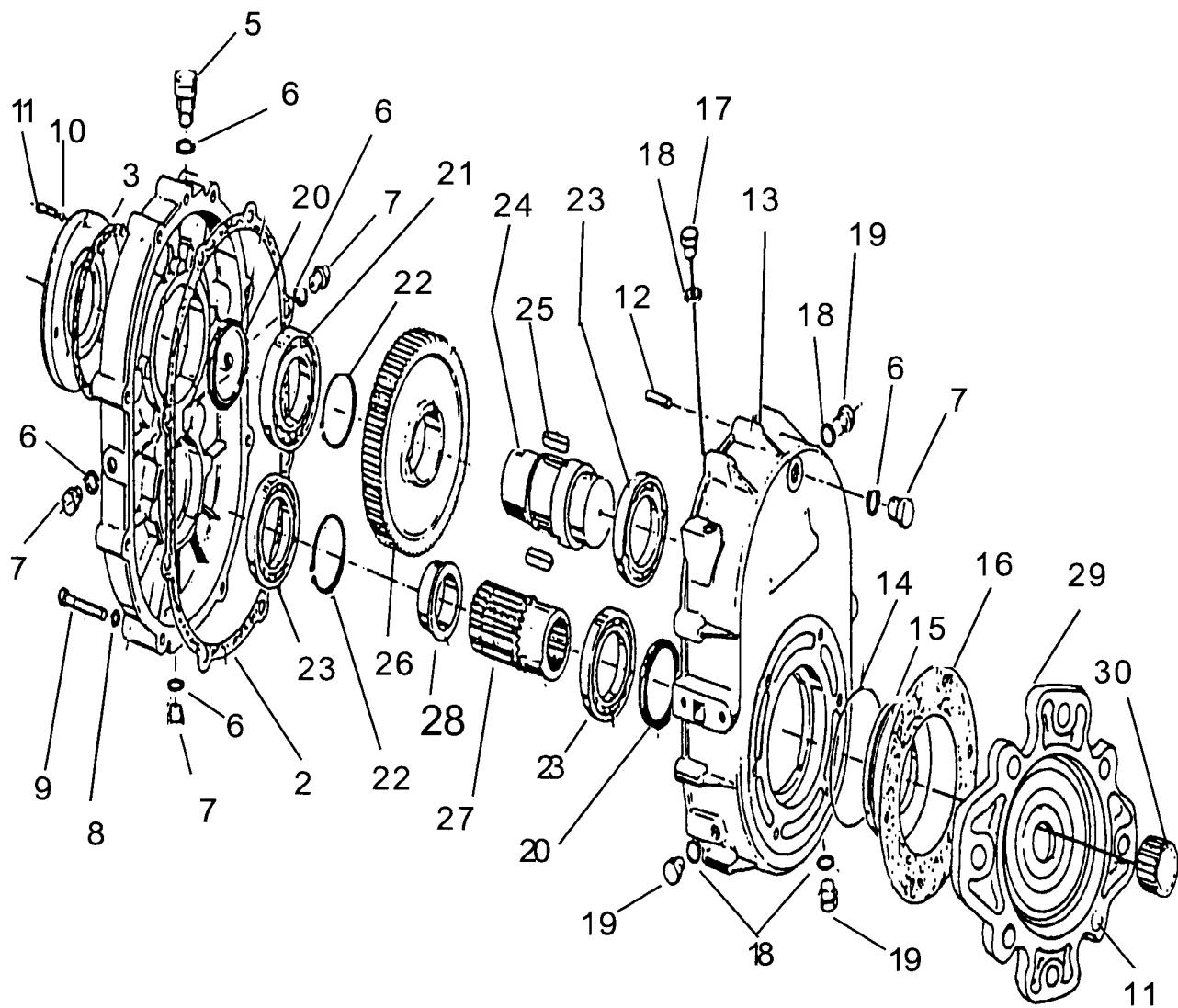
**NOTE:** These Speed Changers have a Cast Aluminum Housing, The 540 RPM has a 1:4 gear ratio and 1000 RPM has 1:2 gear ratio.
