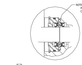
NOTE: FLAT SIDE OF SEAL RETAINER MUST FACE SEAL IN SHAFT END COVER AS SHOWN.
