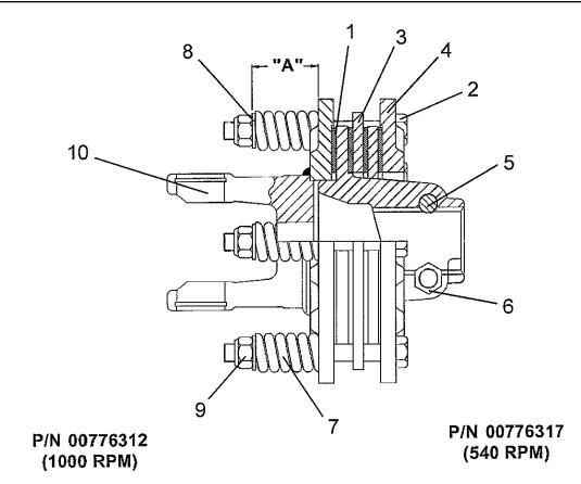
NOTE: "A" = Adjustment Slip Clutch Spring Height
